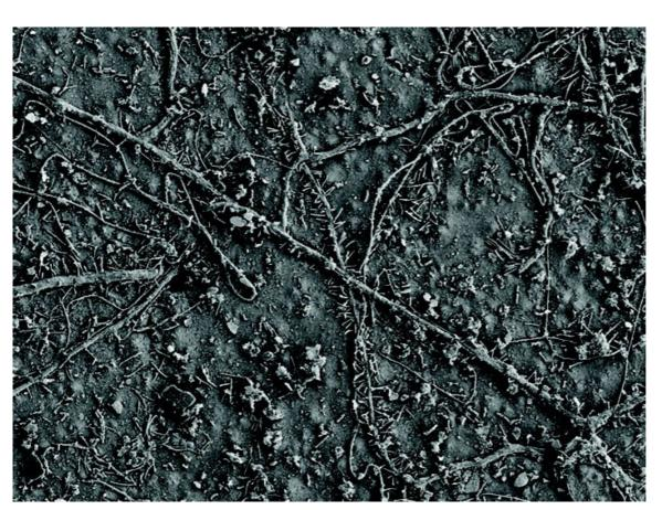
Numerous microbial colonies dot the surface of the biodegradable films, as shown in this scanning electron microscope image.
