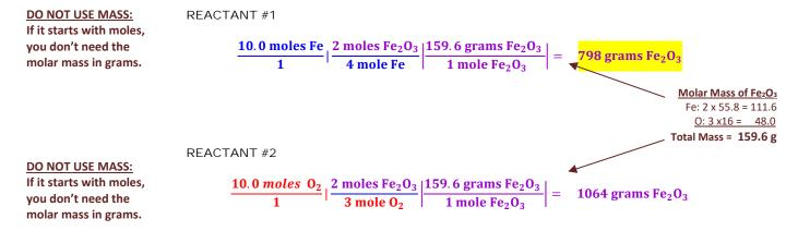
Because it makes less iron III oxide, Reactant #1 (Fe) is the limiting reactant.
