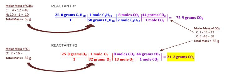
Because it makes less carbon dioxide, Reactant #2 ( $O_2$ ) is the limiting reactant.
