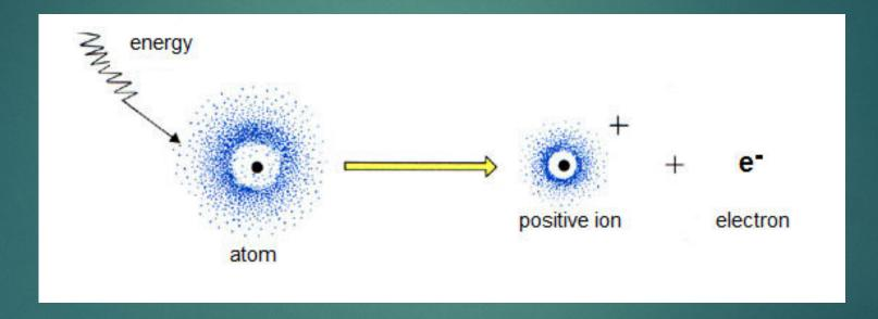
▶ The process of removing an electron is always *endothermic*.
